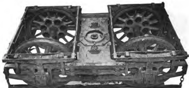
Fig. 4651. Top View of Truck Without Motors. Westinghouse A. C. Electric Locomotive.
